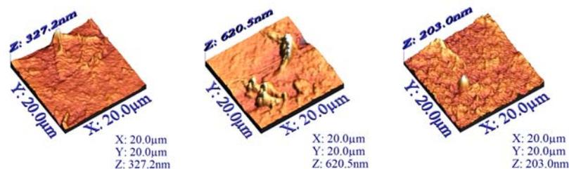
**Figure 3.** Phase transition on combined fullerene graphene systems through the AFM technique. (a) Left - Graphene oxide dissolved in water – “Graphenea” in an isopropyl alcohol solution. (b) Center - Graphene oxide dissolved in water – “Graphenea” in ethylene glycol solution. (c) Right - Graphene oxide dissolved in water – “Graphenea” in water
