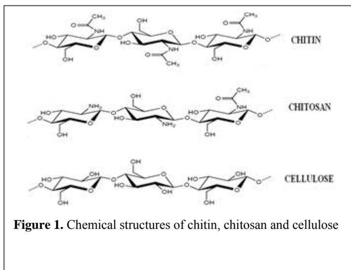
**Figure 1.** Chemical structures of chitin, chitosan and cellulose
