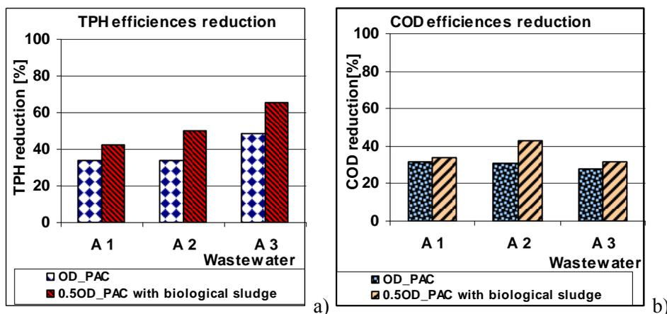
**Figure 1.** Reduction efficiency of the organic load of wastewater when using the optimal dose of PAC, of the reduced dose of PAC and of sewage sludge as aids
